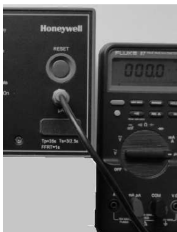
Fig. 4-3: Measuring flame signal with multi meter ( \mu A range selection) using a jack plug.
