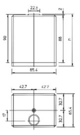
h: The dimensions differ according to the type of socket: 95 with socket A 99 with socket B 98.3 with socket N
