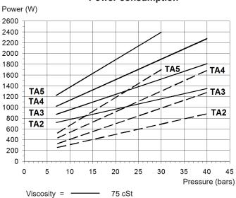
Viscosity = 75 cSt 5 cSt - Rated speed = 2850 rpm
