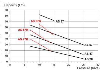
5 cSt - Rated speed = 2850 rpm Viscosity = 1,8 cSt
